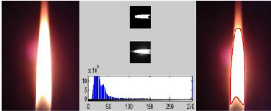
Figure 7. Tested candle flame image and its histogram
