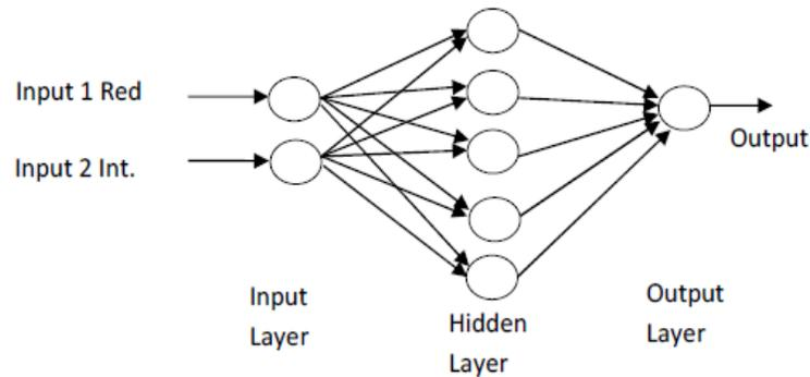
Figure 2. Structure of a Multilayer Neural Network
