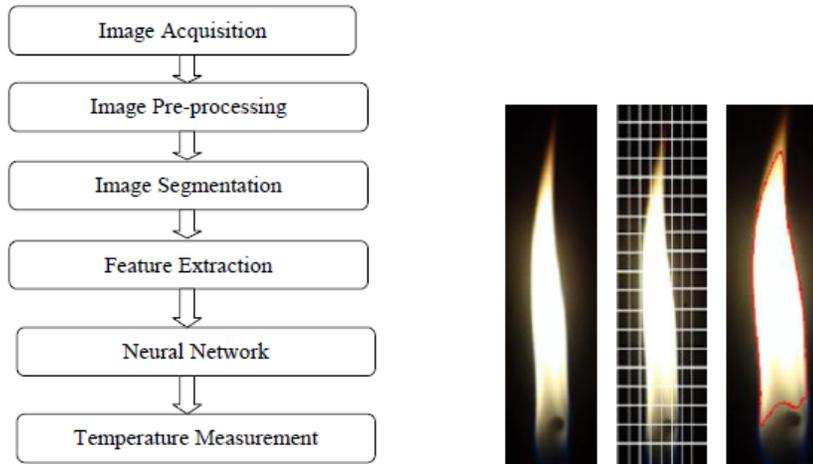
Figure 3. System Flow Chart Figure 4. Original flame & segmentation
