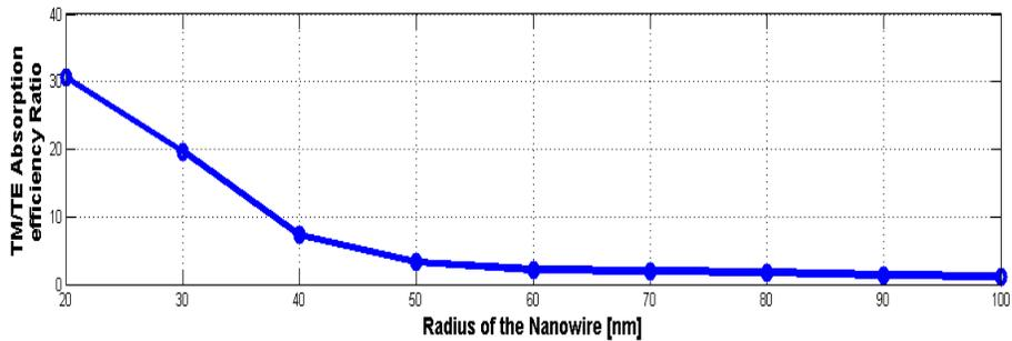
Figure 5: TM/TE absorption efficiency ratio versus radius of the nanowire for 600nm wavelength.
