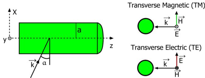
Figure 2: Schematic diagram of the nanowire and directions of transverse magnetic and electric fields.
