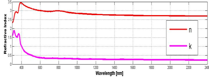
Figure1: Complex Refractive Index of the CdTe. Real part of refractive index is denoted by  $n$  and complex part is denoted by  $k$ .
