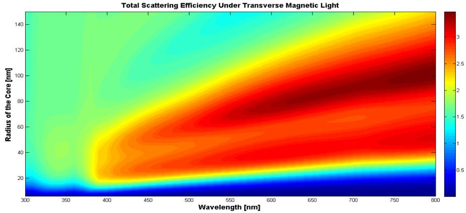
Figure 9: Total scattering efficiency for Transverse Magnetic Wave for various wavelength and radius of the core.
