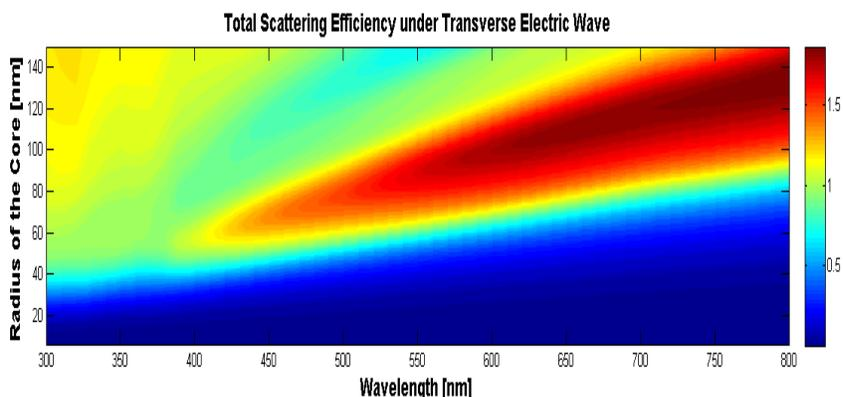
Figure 10: Total scattering efficiency for Transverse Electric Wave for various wavelength and radius of the core.
