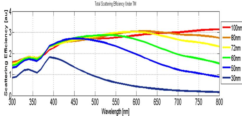
Figure 7: Effect of Radius on Scattering Efficiency for various diameters of the nanowires under Transverse magnetic field for perpendicular Illumination.
