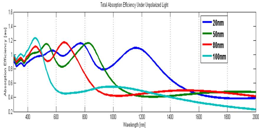
Figure 3: Multiple Peaks resulting from leaky mode resonances for various nanowire radii.
