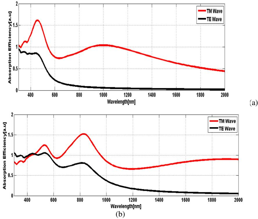
Figure 4: Effect of Transverse Magnetic and Transverse Electric wave on absorption Efficiency for (a) 50nm and (b) 100 nm.
