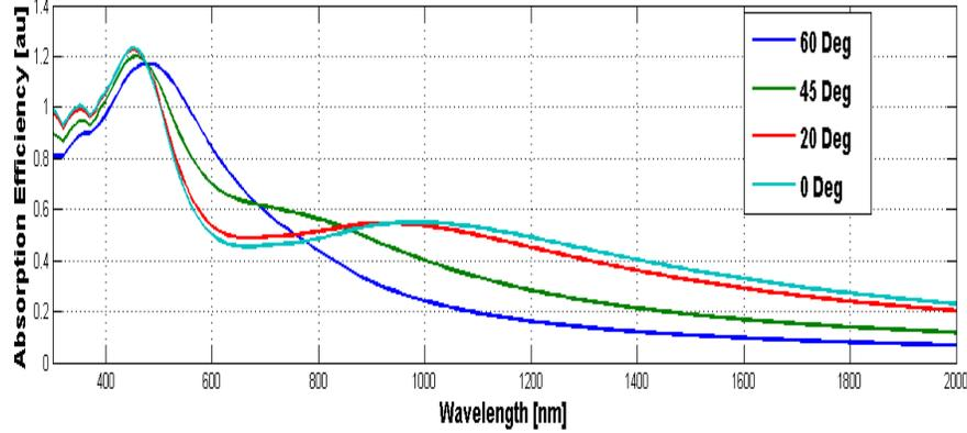
Figure 6: Variation of Absorption efficiency with angle of incidence.
