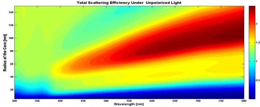
Figure 8: Total scattering efficiency for Un-polarized light for various wavelength and radius of the core.
