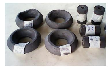
Figure 1. Fabricated MRE Bushings
