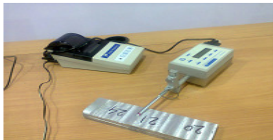
Figure 2 Surface roughness tester and its working
