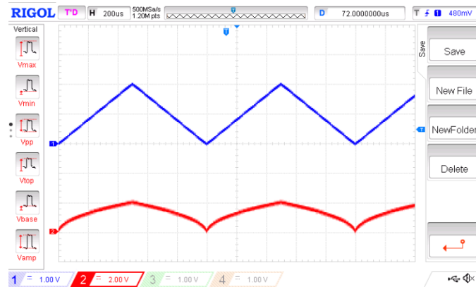
Figure.7. The input signal and output signal where the bias current value is 200 \mu A .
