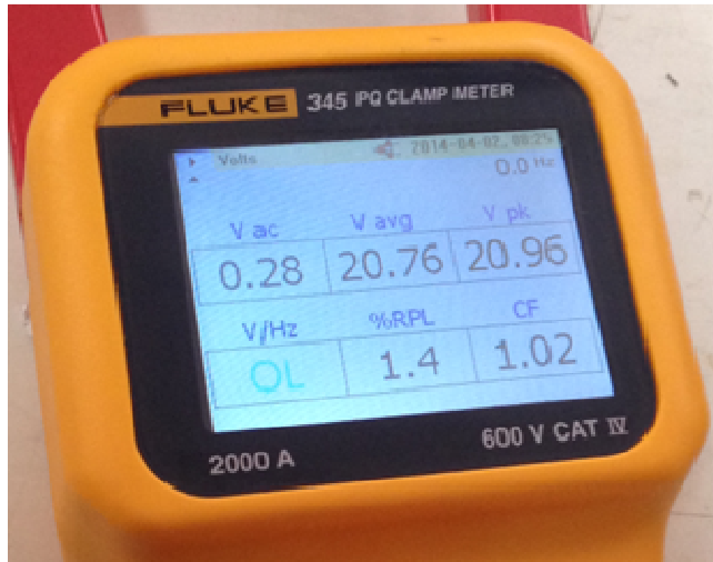
Fig.9 Output voltage ripple of IBC with RCN using PQ Analyser
