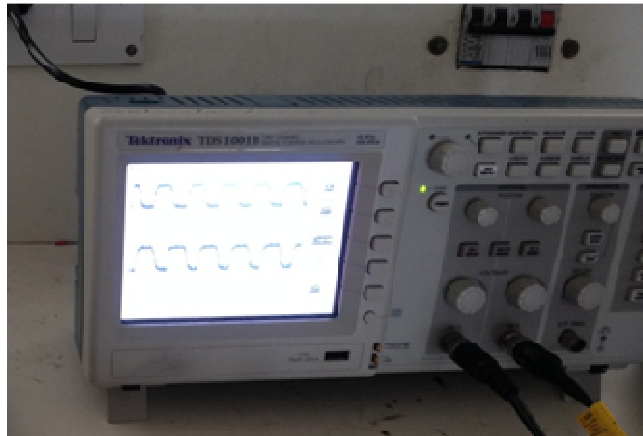
Fig.7 Gate pulses phase shifted by 180^\circ
