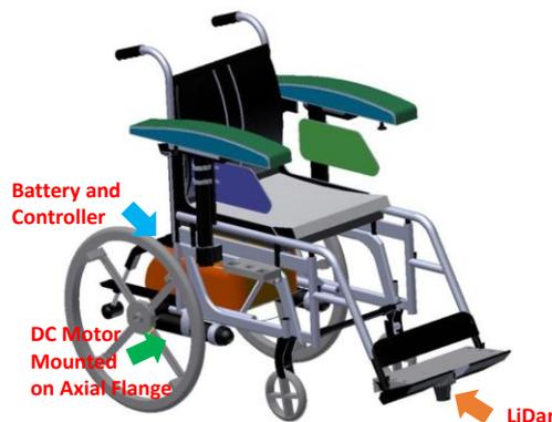
Figure 1. CAD of the adds-on modules of the proposed robotic wheelchair
