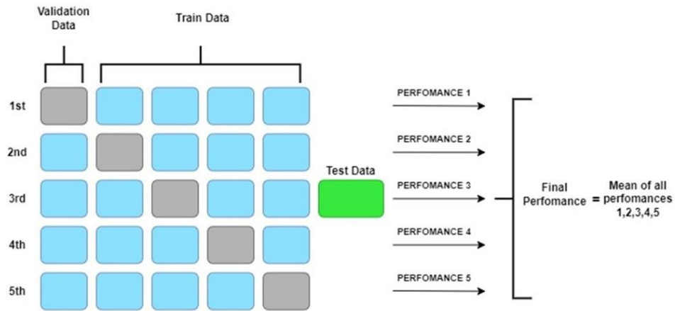
Fig. 4. Cross-validation with five levels of replication. The outcomes of five iterations are the average of all performances.
