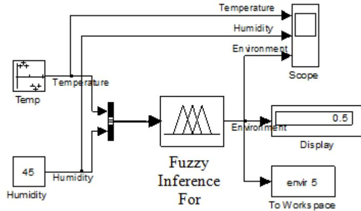
Fig. 5: Simulink Model for Environment Condition determination with constant Humidity
