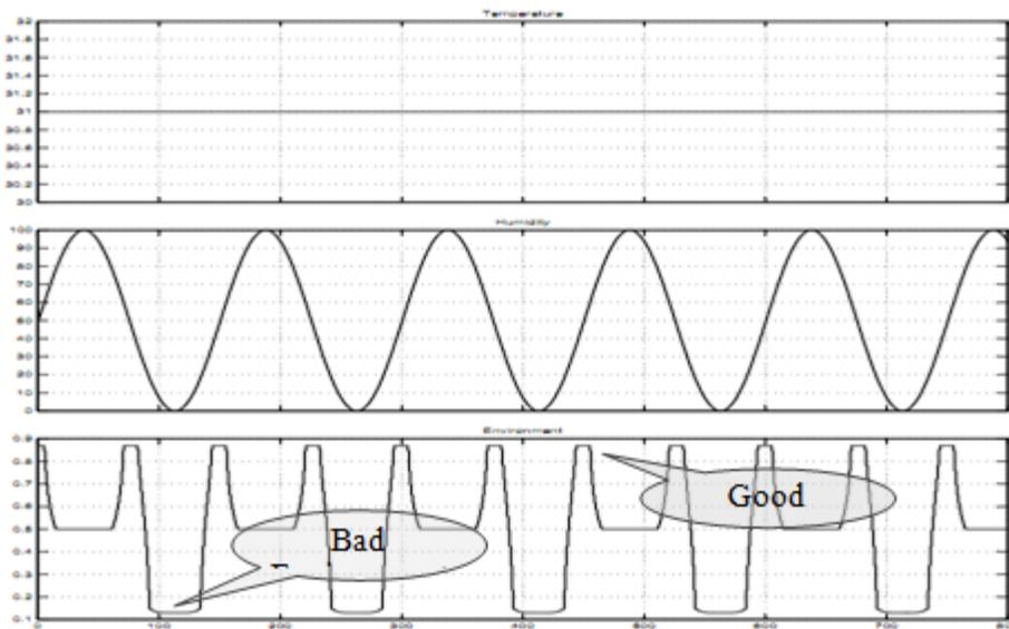
Fig. 11: Simulation results with Temperature constant for Environment determination
