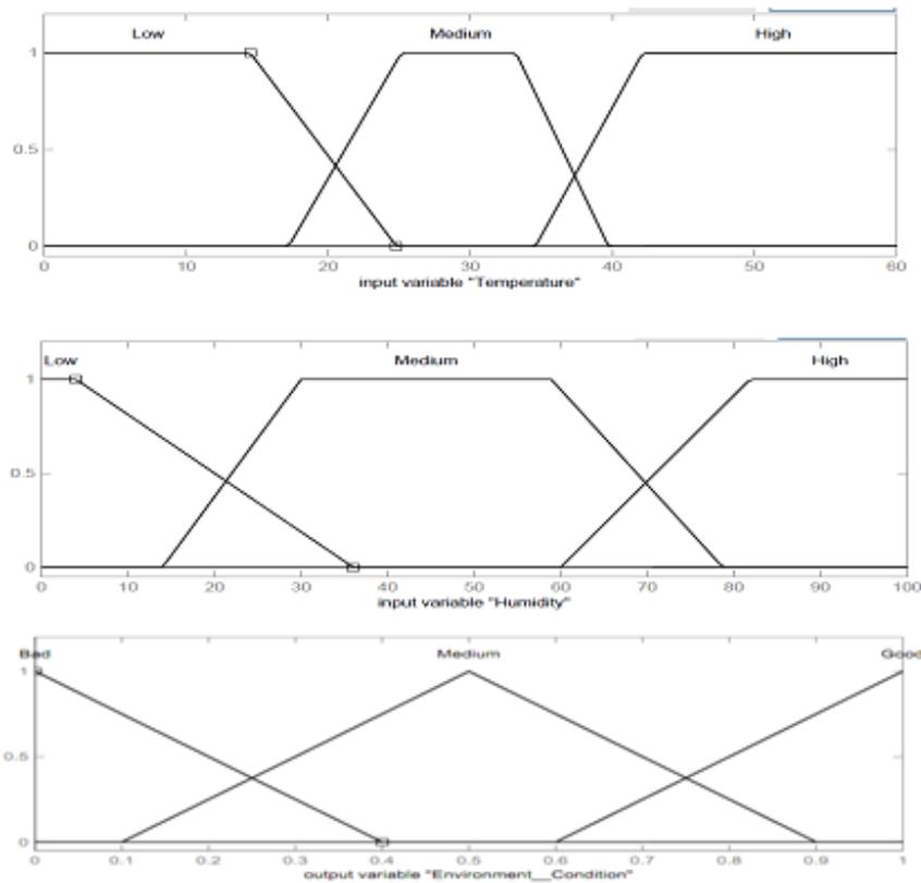
Fig. 3: Membership functions of Temperature, Humidity and Environment Condition
