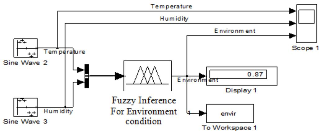
Fig. 6: Simulink Model for Environment condition determination with variable input
