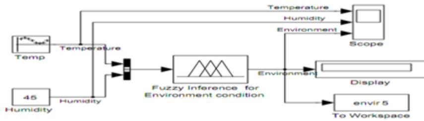
Fig. 12: Simulink Model for Environment Condition determination with constant Humidity
