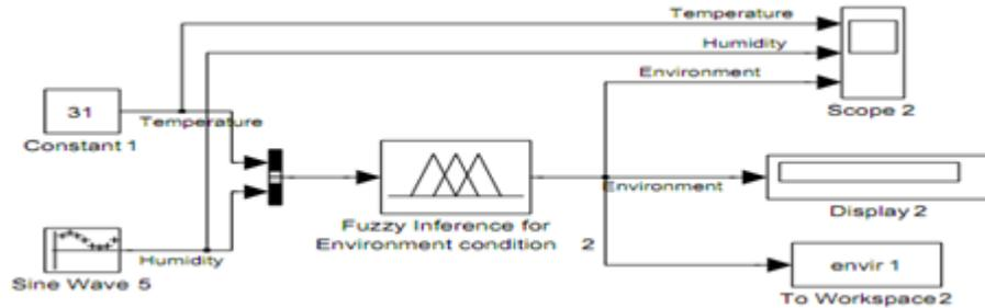
Fig. 10: Simulink Model for Environment condition determination with constant temperature
