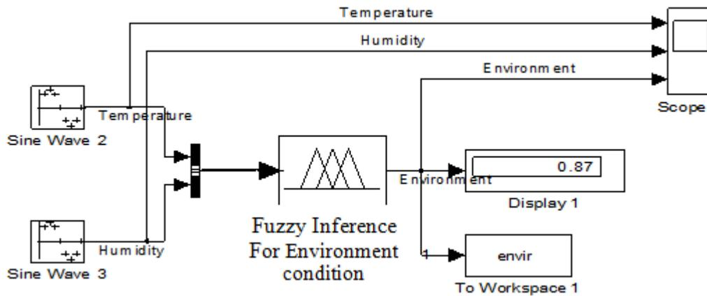
Fig. 6: Simulink Model for Environment condition determination with variable input
