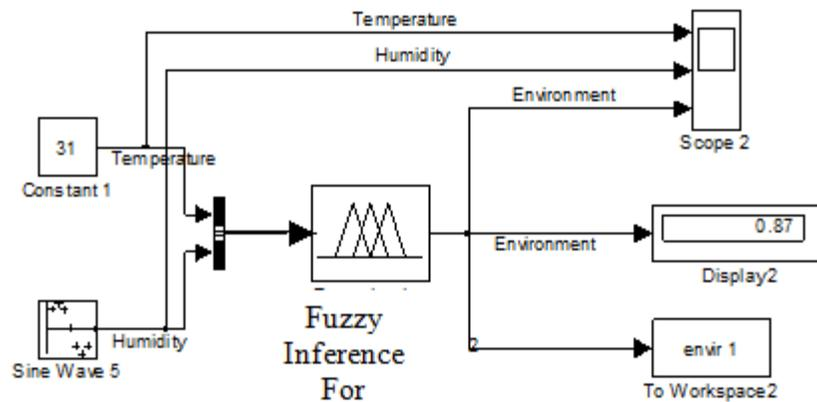
Fig. 4: Simulink Model for Environment condition determination with constant temperature
