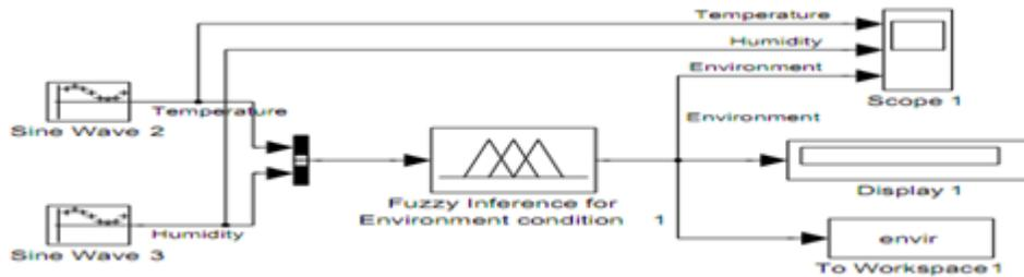
Fig. 14: Simulink Model for Environment condition determination with variable input
