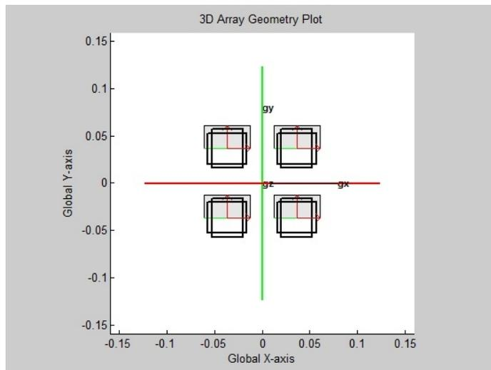
Fig. 3. 3D Geometry of a 2 x 2 microstrip antenna
