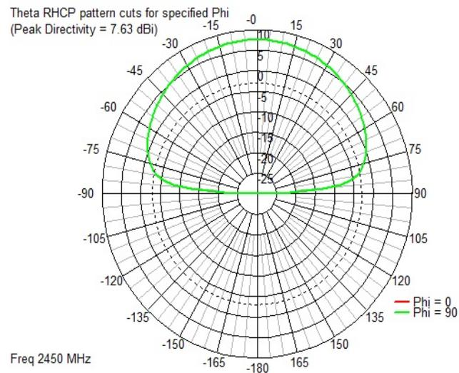
Fig. 5. Radiation pattern for a single microstrip patch antenna
