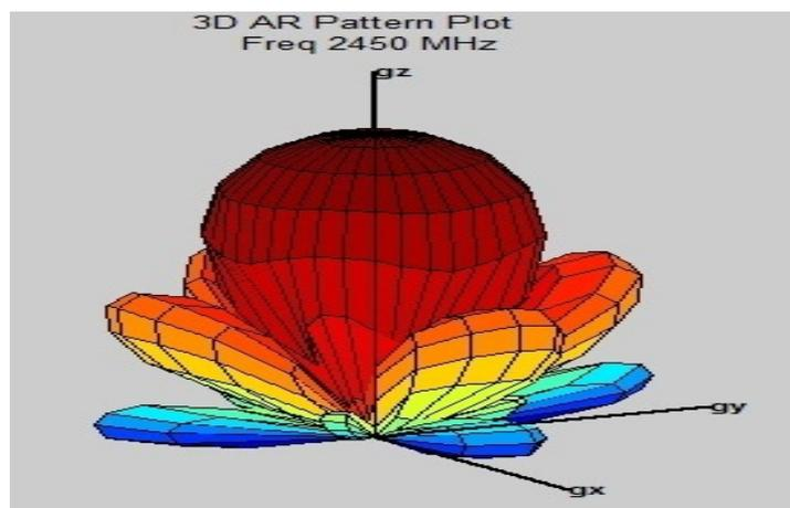
Fig. 10 3D radiation pattern of a 4 x 4 microstrip antenna
