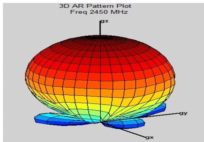
Fig. 9. 3D radiation pattern of a 2 x 2 microstrip antenna
