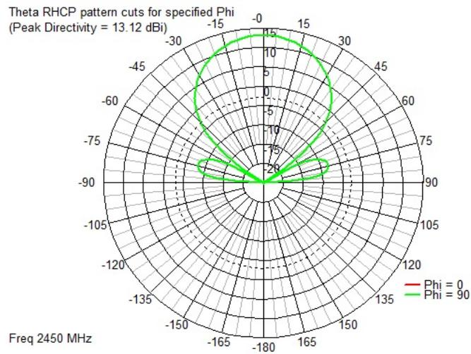
Fig. 6. Radiation pattern for 2 x 2 microstrip patch antenna
