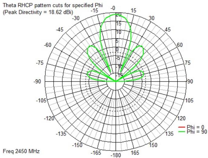
Fig. 7. Radiation pattern for 2 x 2 microstrip patch antenna
