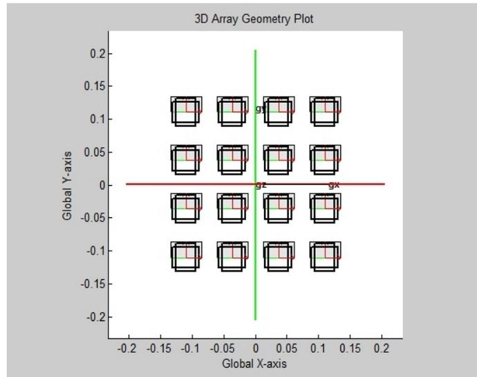
Fig. 4. 3D Geometry of a 4 x 4 microstrip antenna
