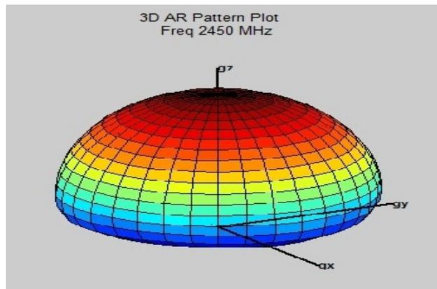
Fig. 8. 3D radiation pattern of a single microstrip antenna
