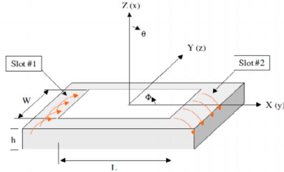
Fig. 1 Geometry of rectangular microstrip patch
