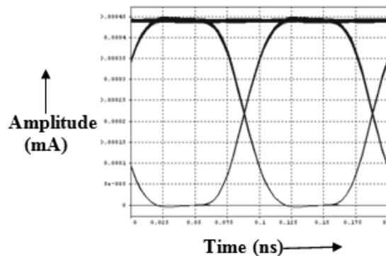
Figure 3.6: EYE Diagram of received signal
