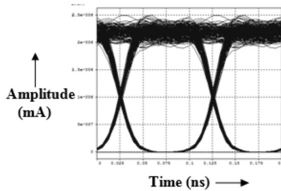
Figure 2.3: EYE Diagram after compensation
