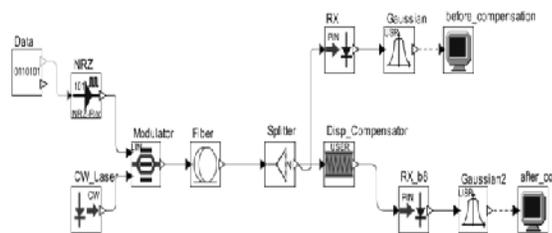
Figure 2.1: Block Diagram of FBG
