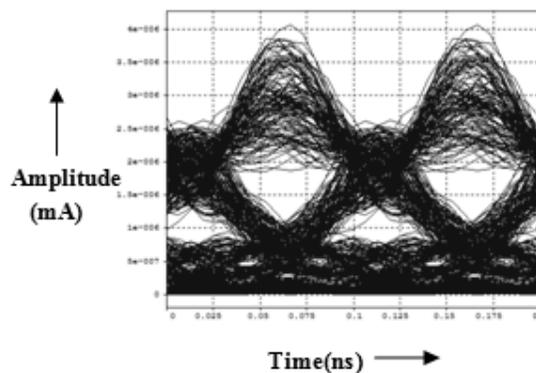
Figure 2.2: EYE Diagram before compensation
