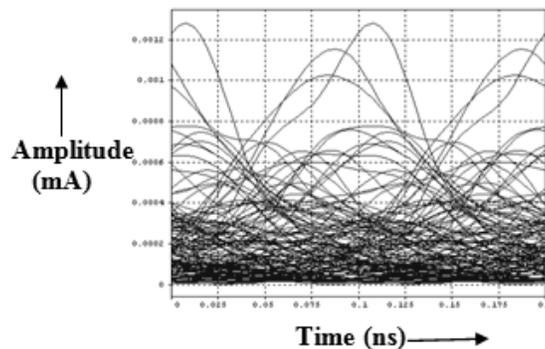
Figure 3.4: EYE Diagram after 1000km\_b15
