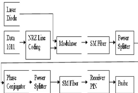
Figure 3.1: Schematic setup for dispersion compensation by phase conjugation
