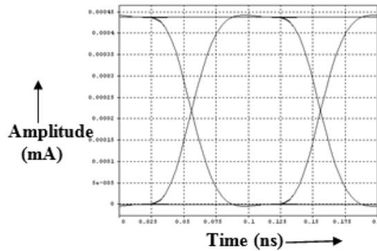
Figure 3.3: EYE Diagram of transmitted signal
