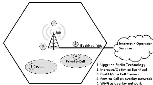
Fig 1. Backhaul and Radio are two choke points.
