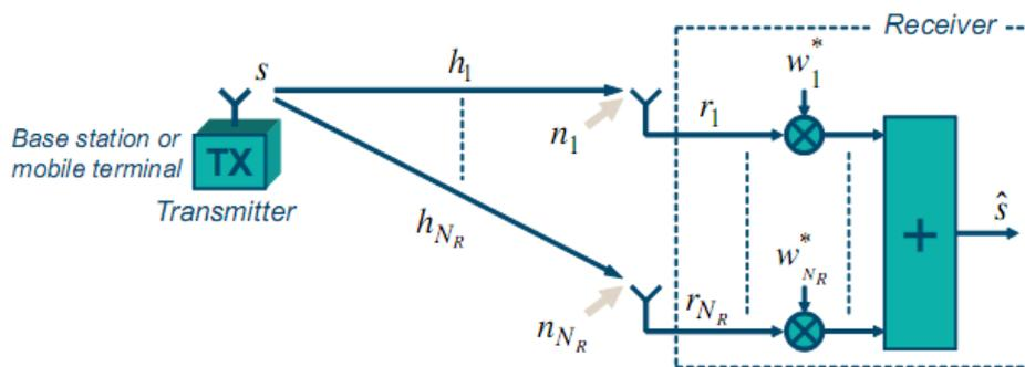
Figure 3. Linear receive-antenna combination.
