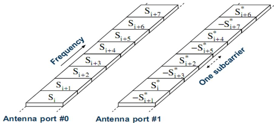
Figure 4. Transmit diversity for two antenna ports – SFBC.
