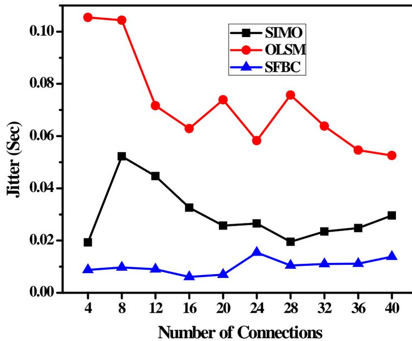
Figure 8. Jitter performance for varying number of connections
