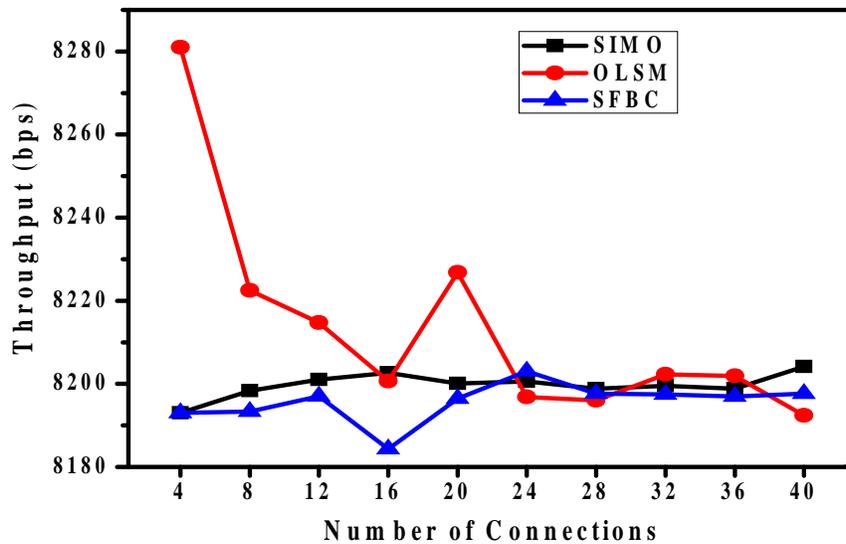
Figure 6. Average throughput performance for varying number of connections
