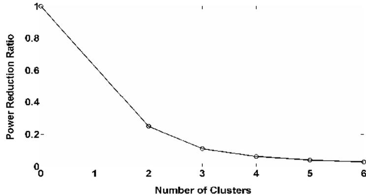
Figure 6: Power reduction ratio vs number of clusters in the axis of transmission
