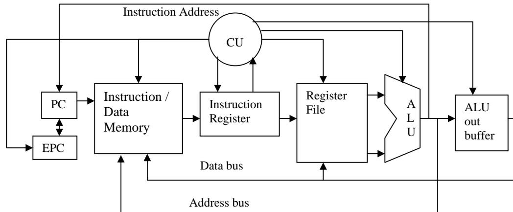
Figure 1: Developed Soft Core Processor Architecture for RR- Node
